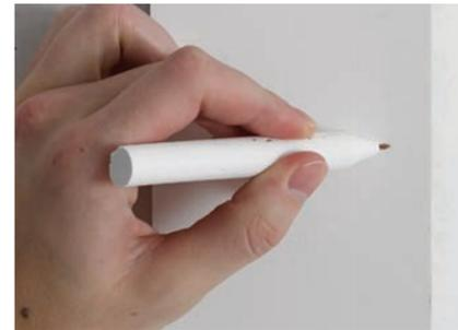
Use AZEK Nail Eraser to smooth surfaces marked by nails with small surface heads.
